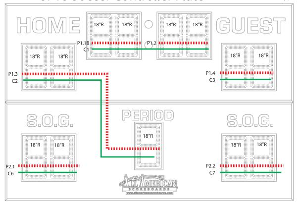
Power Supply Outputs (Full Brightness & Full Digits): P1.1≈3.82A P1.2≈2.38A P1.3≈3.57A P1.4≈2.38A P2.1≈2.38A P1.2≈2.38A
