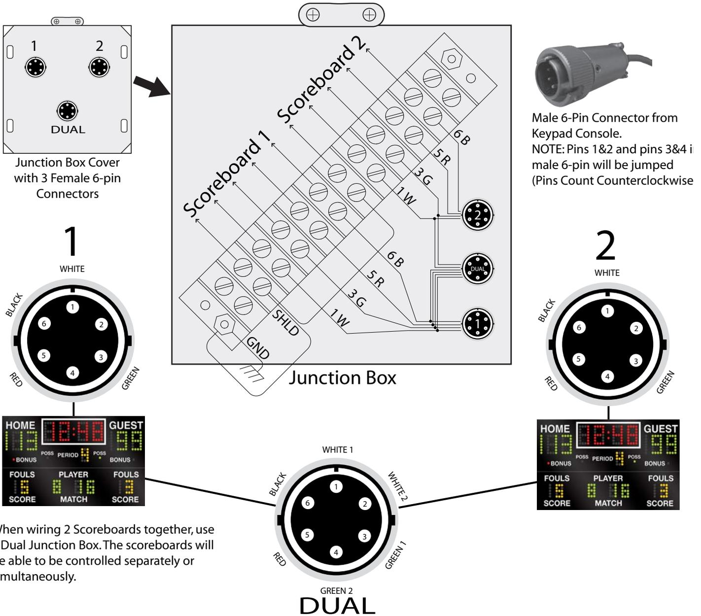
When wiring 2 Scoreboards together, use a Dual Junction Box. The scoreboards will be able to be controlled separately or simultaneously.
