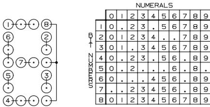
MICROPROCESSOR 4 X 7 (8 BIT) LAMP PATTERN
