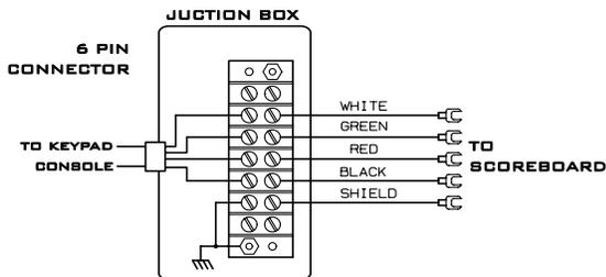
Figure 3: Junction Box (Cable Hard-wire System only)
